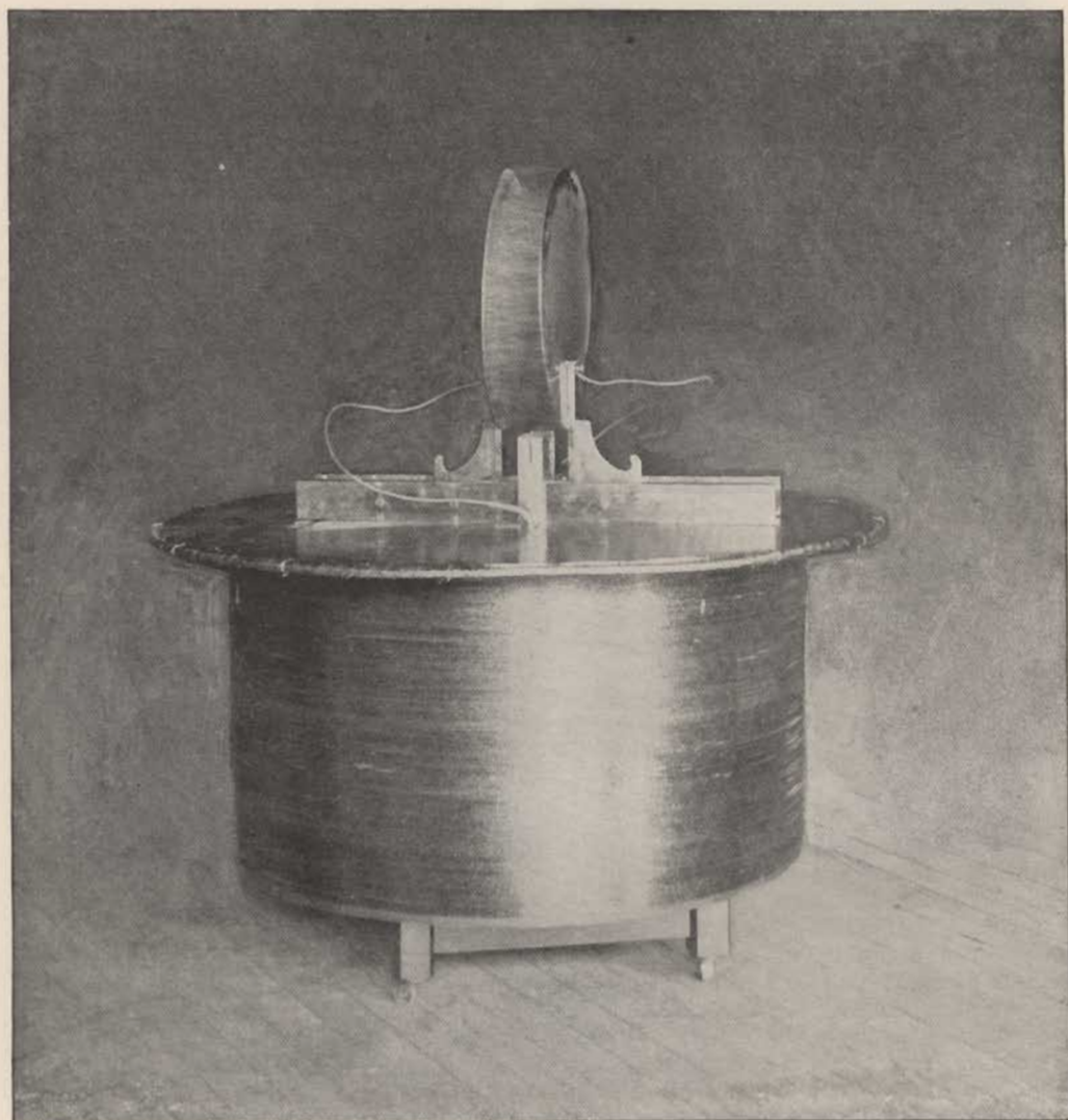
FIG. 9. EXPERIMENT SHOWING PLAY OF ELECTRIC SPARKS BETWEEN CONDENSER PLATES, PRODUCED BY ELECTRIC CHARGE. THE COIL, STANDING IN THE CENTER OF A LARGE ROOM, IS UNCONNECTED WITH THE ENERGIZING CIRCUIT. (FROM FLASH-LIGHT PHOTOGRAPH.)
